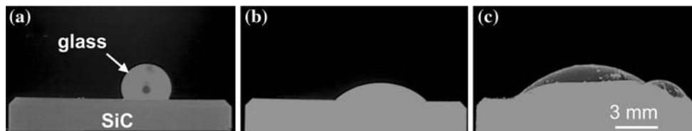
Fig. 4 Droplet profiles during a wetting experiment of a 23CaO–15Al 2 O 3 –62SiO 2 (wt%) glass on sintered SiC under air at T = 1590 °C after 10 s (a), 90 s (b) and 1,800 s (c) of spreading. t = 0 is taken to be complete melting of the glass
